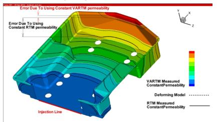
**Figure 1**: Comparison of predicted flowfronts using the RTM filling simulation with permeability measured with VARTM methodology (colour contours), permeability measured with RTM experiment (solid lines) and fully deformable model (dashed lines). Maximal change of preform thickness set to 10%.
